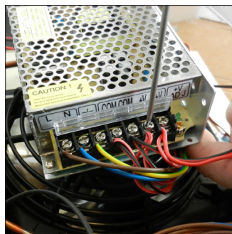
D2. Disconnect the power supply from the wiring
