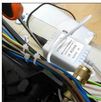
F1. Unscrew the screws holding the receptor to the tank
