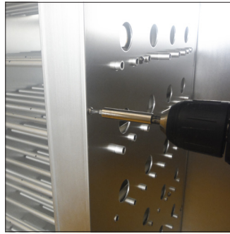
C2. Unscrew all the bolts and remove central alluminium pannel right side
