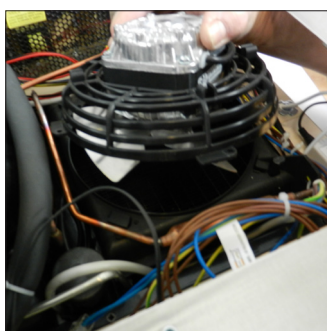
L2. Extract the fan rotating it counterclockwise
