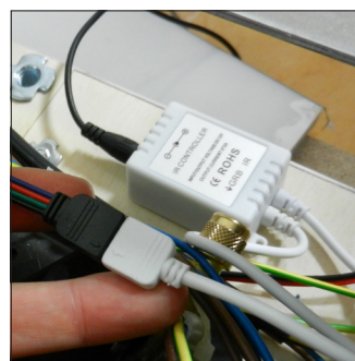
F3. Reposition the new receptor and connect the power supply and the LEDS
