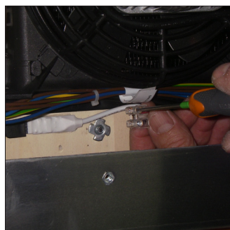
F4. Disconnect the power supply wires and the leds connector
