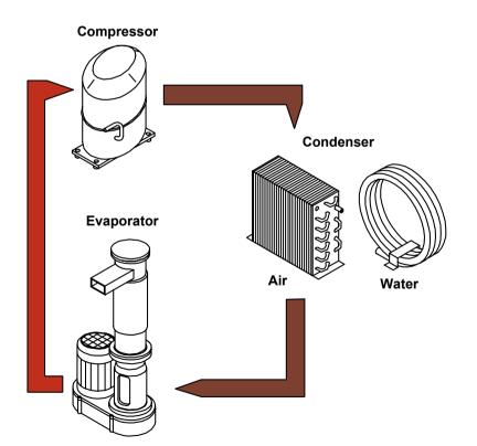
Each ice maker uses the properties of compression and expansion of the liquefiable gases; its main principle is that each change of bodies state is got by producing or absorbing heat.
