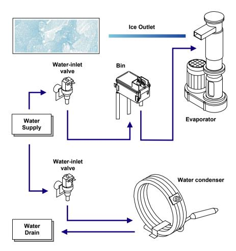
The circuit of water supply of the bin and the evaporator is on all machines of the 'GB'-line; the second circuit is, on the contrary, only on water-cooled versions.
