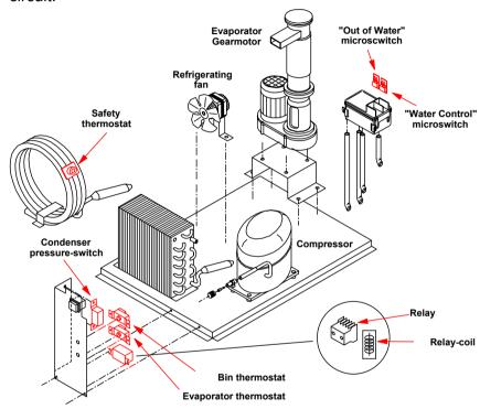
The relay gives power to the Compressor, the Refrigerating fan and the Water-inlet valve for the water-condenser (see previous diagram).
