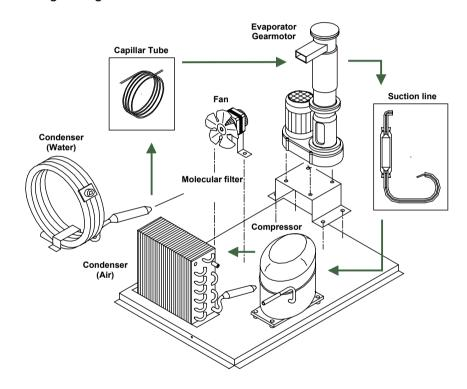
The refrigerating circuit includes the equipments set that permit the compression and the expansion of the refrigerating gas, by producing the cold necessary to get ice.
