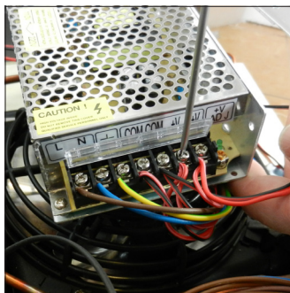
E5. Disconnect the broken LED strips from the power supply
