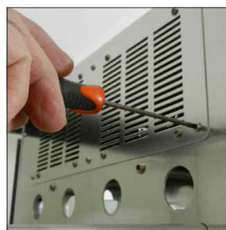
I3. Reconnect the fans, tighten them and reassemble the carter
