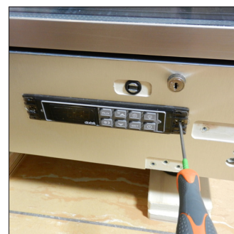
G4. Install the new thermoregulator and apply the cover lid fixing one spring at a time
