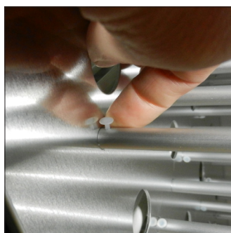
A1. Extract the plastic clip from the right hand side on the alluminium rods
