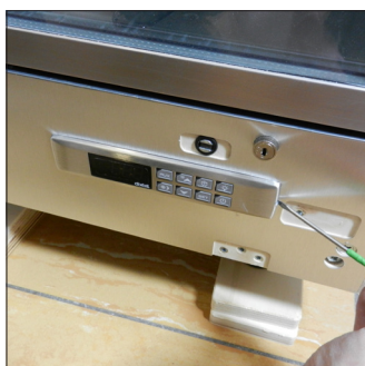
G1. Extract the metal cover unfastening the lateral spring (use a small flat screwdriver)
