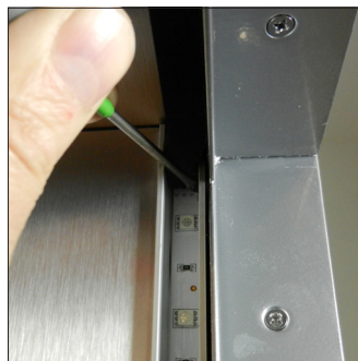
E6. Extract the broken LED strips from the guide, operating with a screwdriver
