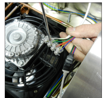
E4. Connect the new LEDs to the receptor cable as they were before matching the colors
