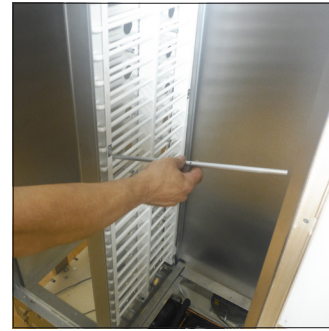
C3. After removing all the plastic clips extract all the aluminium rods from the right compartment of the unit display
