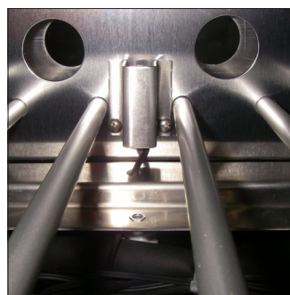
H3. Fasten the probe and carter passing along the lead from the suitable hole on the bottom crossbeam
