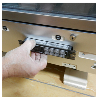
H1. After extracting the thermoregulator disconnect the probe from the terminal
