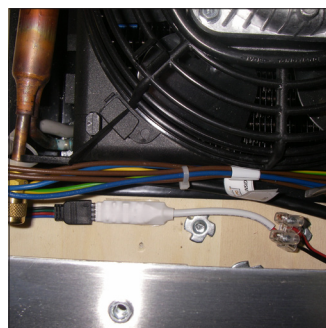
F5. Reposition the new receptor and reconnect
