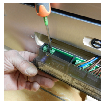
H4. Reconnect the probe to the thermoregulator
