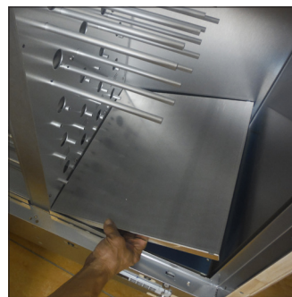
A3. Remove the alluminium panel
