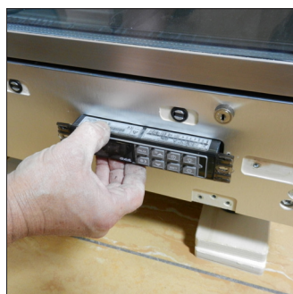
G2. Unscrew, extract the thermoregulator and disconnect the cables
