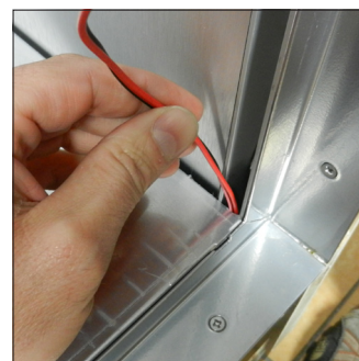
E3. Insert the new LED strips in the aluminium profiles and extract the 4 cables from the holes in the basin
