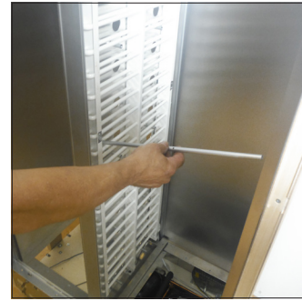
C3. After removing all the plastic clips extract all the alluminium rods from the right compartment of the unit display
