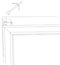
8. Tighten the top hinge pin.
