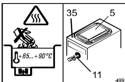
**RISCHIO RESIDUO: IL PRODOTTO, DURANTE IL TRATTAMENTO DI PASTORIZZAZIONE, VIENE PORTATO AD ALTE TEMPERATURE (+65...90°C). IL CONTATTO CON ESSO, CON IL COPERCHIO [5], CON IL RUBINETTO [11] E CON IL PIANO DELL'APPARECCHIO [35] PUÒ CAUSARE GRAVI LESIONI. SI RACCOMANDA PERTANTO DI:**
