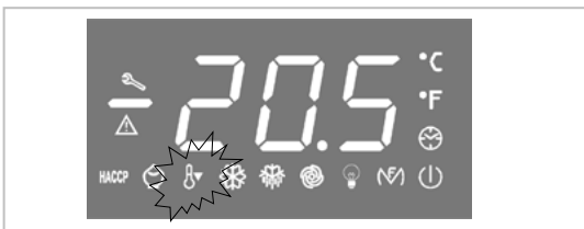
This LED indicates the activation of the OVER COOLING function
