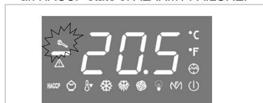
THE LED lights require cleaning of the condenser filter.
