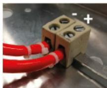
The wire marked with 2 cable ties is the minus terminal; the wire marked with 1 cable tie is the plus terminal.
