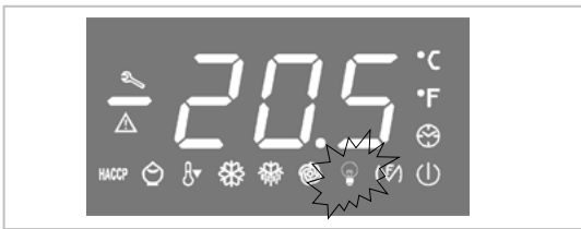
This LED indicates the state (on or off) of the LIGHT
