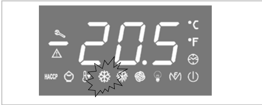
This LED indicates the state (on or off) of the COMPRESSOR
