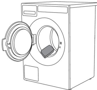
Connect the washing machine to the power mains and run the dedicated drum cleaning program. See chapter "WASHING PROCESS; STEP BY STEP (1-8)" /STEP 5: CHOOSE THE PROGRAM.
