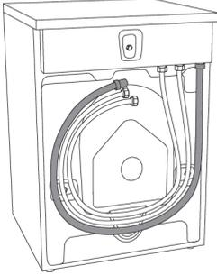
Upon delivery, the appliance has a drain hose attached. This drain hose must be connected to a drain. Drain hose can also be attached to a wall drain with a trap; such trap should be properly installed to allow cleaning. The height of the drain should be 600–900 mm above the floor. The lower position (600 mm) is always recommended. Make sure the drain hose is not clipped or bent.
