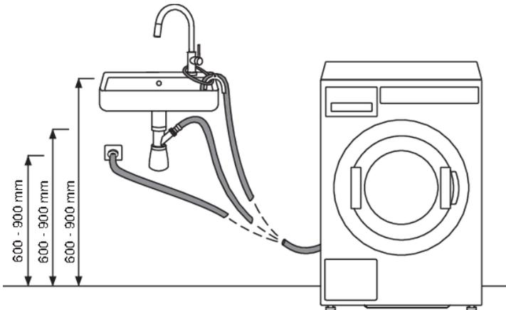
Drain hose can also be connected directly to the washbasin drain via a siphon. In this case, the hose, should be 600–900 mm above the floor. Internal hose diameter should be at least 18 mm.
