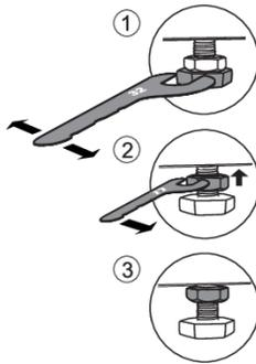
1. Level the washing machine in longitudinal and traverse direction by rotating the adjustable feet (using a No. 32 spanner). The feet allow levelling by +/- 1 cm.
